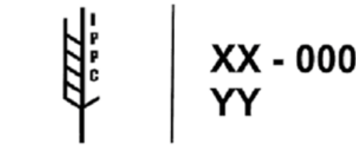
XX represents the ISO country code. 000 represents the unique number assigned by the national plant protection organization. YY represents either HT for heat treatment or MB for methyl bromide fumigation.
